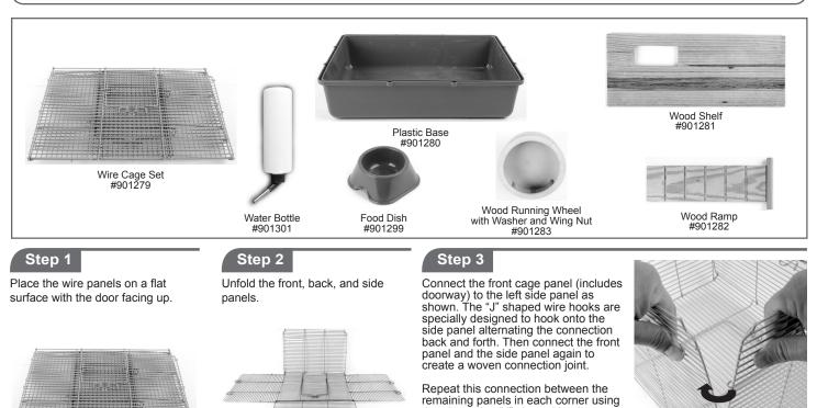
HINT: Start by attaching bottom "J" hook and move up and attach top "J" shaped hook last.
