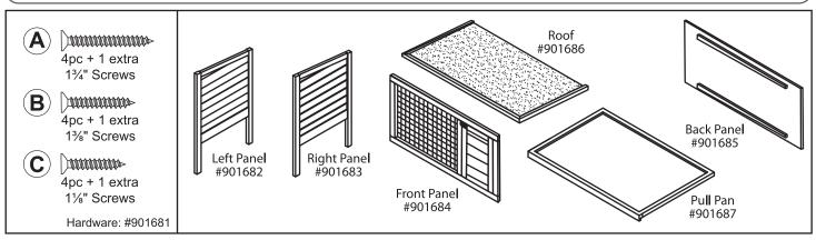
Attach the Right Panel and the Left Panel to the Front Panel using  $4 - 1\frac{3}{4}$ " screws (A).
