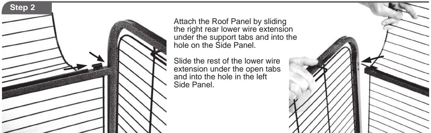
Attach the Roof Panel by sliding the right rear lower wire extension under the support tabs and into the hole on the Side Panel.
