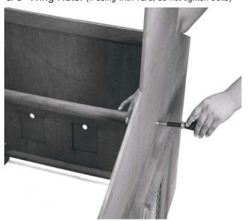
Before installing both side lids, insert Roost & secure each side with 3/4" Bolts.
