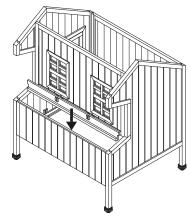
Position the Rooftop in place and attach with 8 – 1 3/8" (C) screws. Attach the molding to the front using 2 – 1" screws. Place the Ridge Cap on top of the roof and attach with 4 – 1" screws (D). Attach Handles to front of hutch using 4 – 1" screws (D). Connect Nest Box Door to top of nest box area of the hutch using 4 - 2/3" (E) screws on the pre-attached hinges on the door.
