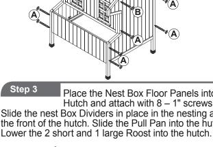
Lower the Nest Box Floor Support into the front of the hutch and slide in place in the notches on the inside of the Side Panels.
