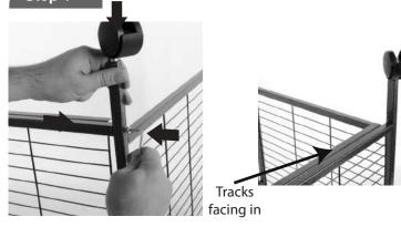
Insert a non-locking Wheel into the Right Side Panel so the holes line up, then insert Bolt. Align the hole in the bottom of the Back Panel with the hole in the Side Panel that you just placed the Bolt through. Using the Hex Wrench, screw in the bolt through the Side Panel and into the Back Panel; repeat for the opposite Side Panel making sure the tabs face towards the outside and the tracks face towards the inside of the cage.
