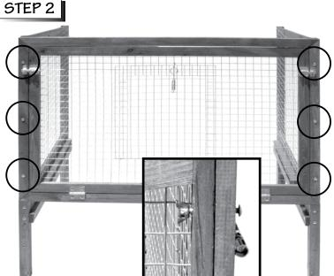
Fasten Side Panels **(B)** to Front Panel **(C)**. Use **6**- 2" Bolts and **6**- Wing Nuts.
